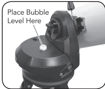
FIGURE 2-5 Leveling the Base
