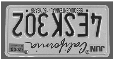
LCM 76/114 – UPSIDE DOWN IMAGE, AS VIEWED WITH THE EYEPIECE DIRECTLY IN TELESCOPE
