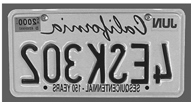
LCM 60/70/80/90 - INVERTED IMAGE WHEN VIEWING WITH THE EYEPIECE STRAIGHT THROUGH (NO DIAGONAL)
